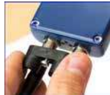
II. Remove Connectors Locking Clip (CLC)
