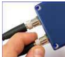
V. Reconnect and manually tighten the new spare unit (Cutter or Control unit)
