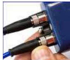
VI. Place Connectors Locking Clip (CLC), and check if CLC locks both connectors
