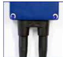
VIII. Check if CLC is closely attached to Main Box (no space between both objects)
