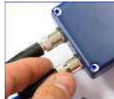
III. Manually unscrew connector
